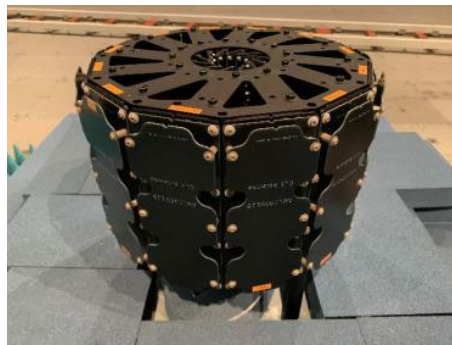
Figure 3.6. HAPS Mobile and SoftBank antenna prototype [6].
